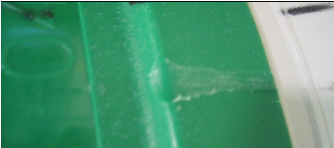
Figure 4: Damage sustained from a horizontal drop, which is the most severe for this type of cylinder. If these marks are found in the cylindrical area or at the joint between the upper and lower casing, the cylinder must be rejected.
