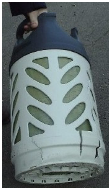
Figure 1: Acceptable outer casing damage caused by abrasion
