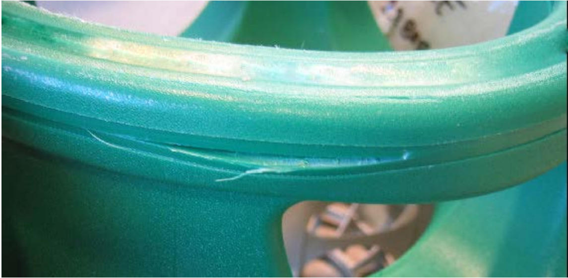
Figures 2 and 3: Unacceptable outer casing damage
