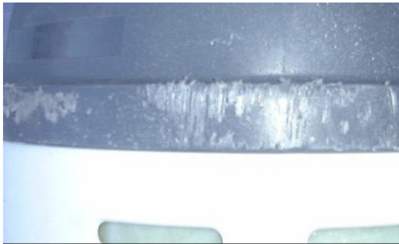
Figure 1: Acceptable outer casing damage caused by abrasion
