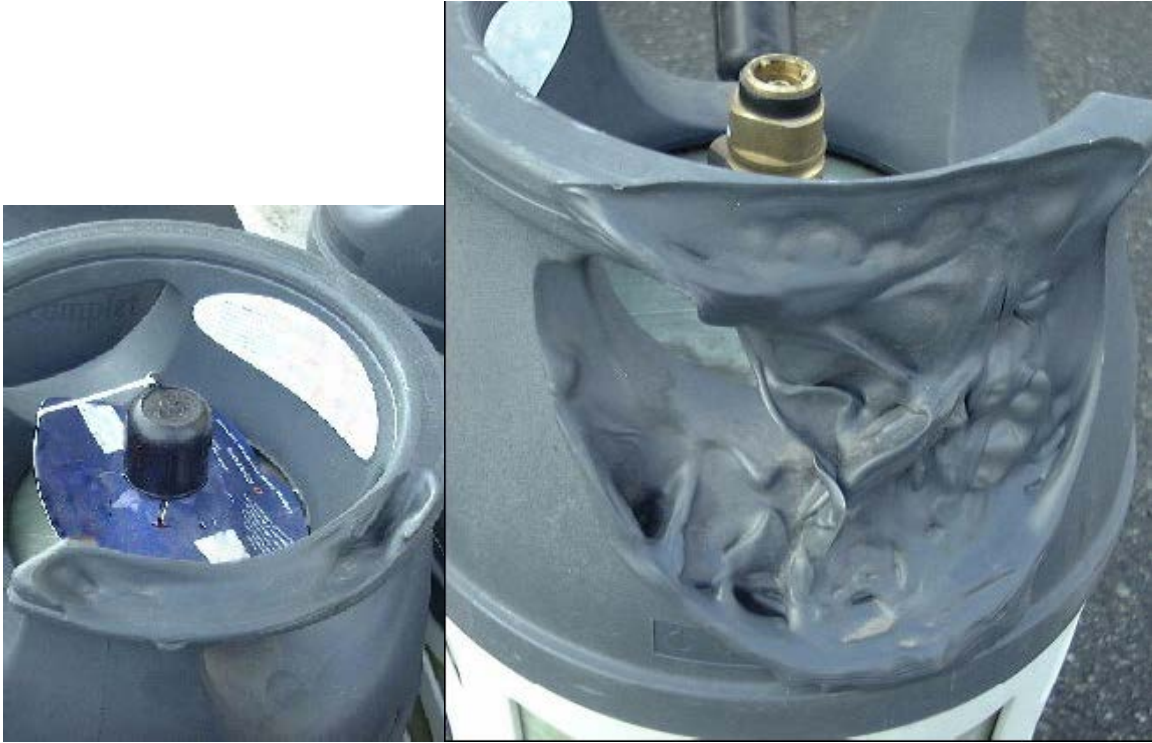
Figures 5 and 6: Unacceptable outer casing heat damage
